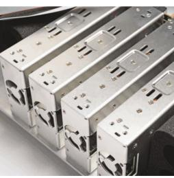
The MCaps are dampened to stop all vibrations. Opposite, the four shielded SMPS power supplies; foam also insulates the four Mundorf chemical capacitors for the power supply from vibration.
