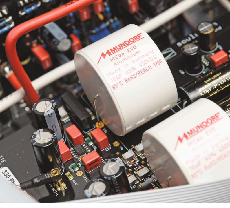
The MC phono board is equipped with German capacitors manufactured by Mundorf et Wima, both quality brands familiar to audiophiles. The 330's audio section is physically separated from the isolated power supply for minimum interference.
