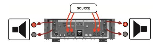
▲ The Source-Out is not attenuated. The full output level of the connected source component will be present at the Source-Out. Amplifiers without volume control function are not allowed to be connected to the Source-Out. Excessive volumes due to inappropriate handling may cause hearing damages or may damage your loudspeakers.
