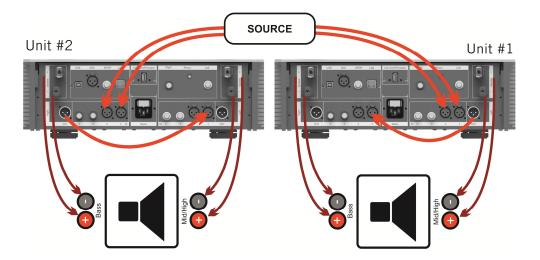
The Source-Out is not attenuated. The full output level of the connected source component will be present at the Source-Out. Amplifiers without volume control function are not allowed to be connected to the Source-Out. Excessive volumes due to inappropriate handling may cause hearing damages or may damage your loudspeakers.
