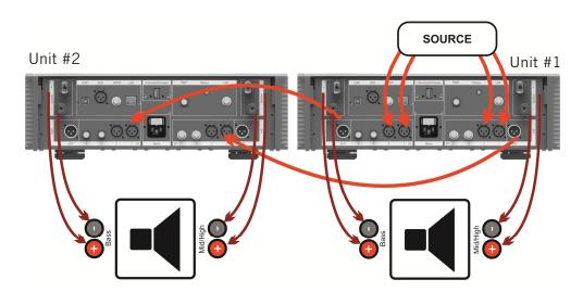
The Source-Out is not attenuated. The full output level of the connected source component will be present at the Source-Out. Amplifiers without volume control function are not allowed to be connected to the Source-Out. Excessive volumes due to inappropriate handling may cause hearing damages or may damage your loudspeakers.
