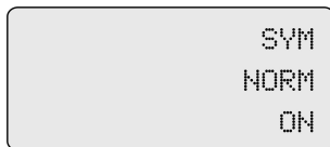
Display in operating condition ON, Mode NORM
