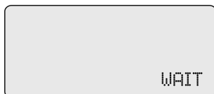
Display after switch on of the mains switch
