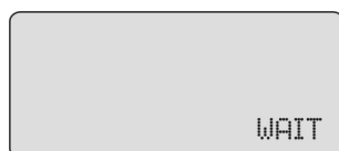
Display after switch on of the mains
