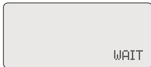
Display after switch in of the mains
